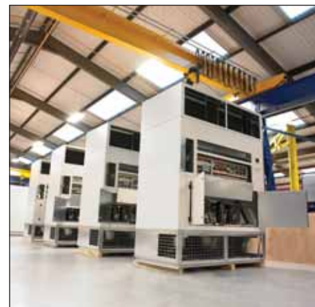
60kW replacement free cooling units being manufactured.
